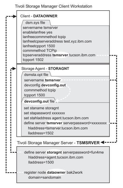
Figure 7. Communications information. Results of Steps 2.1 and 2.2. The passwords are shown as "xxxxxxx" because they are encrypted in the file.
